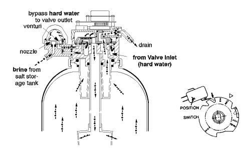
After fill, timer/switch action allows the motor to turn the rotor and disc into BRINING position. Water flow is directed to the nozzle. Suction, created by the nozzle and venturi, draws brine from the salt storage tank and injects it into the resin bed via the bottom distributor. Flow continues out the top distributor and to the drain. Hard water is available at the valve outlet.
